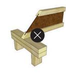
Handling Never lift or move the joist packs by the flanges.
